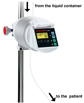
Fig. 13: ASTOTHERM PLUS prepared (without ASTOLINE and without heat protection sleeve)
