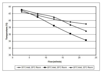
Fig. 3 WP31 outlet fluid temperature at Set temperature 43°C, different room and inlet temperatures
