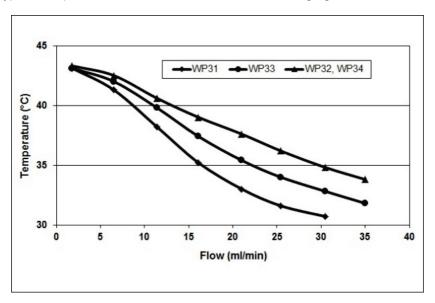
Fig. 1 Typical outlet fluid temperatures at 20°C inlet temperature, set temperature 43°C, PVC
